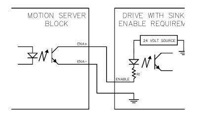
A sinking enable input can be handled with the following hook-up:
