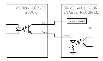
The "Ena +" signal goes to the supply voltage from the drive, and the "Ena -" signal goes to the enable signal of the drive. Current will flow when the controller indicates "enabled" for the drive.
