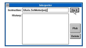
If you configured the XAxis to be a servo motor, the motor should now be displaying stable servo behavior by resisting any applied torques. If the motor is a stepper motor, the amplifier should be enabled and the stepper motor holding position.
